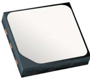
Figure 7. Si7021 with Factory-Installed Protective Cover
