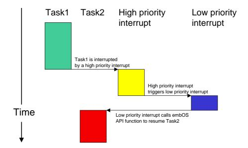
The task 1 is interrupted by a high priority interrupt. This high priority interrupt is not allowed to call an embOS API function directly. Therefore the high priority interrupt triggers a low priority interrupt, which is allowed to call embOS API functions. The low priority interrupt calls an embOS API function to resume task 2.
