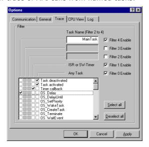
To enable or disable a filter, simply check or uncheck the corresponding checkboxes labeled **Filter 4 Enable** to **Filter 0 Enable**.
