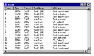
Every entry in the **Trace list** is recorded with the actual system time. In case of calls or events from tasks, the task ID (**TaskId**) and task name (**TaskName**) (limited to 15 characters) are also recorded. Parameters of API calls are recorded if possible, and are shown as part of the **APIName** column. In the example above, this can be seen with OS\_Delay(3). Once the trace buffer is full, trace is automatically stopped. The **Trace list** and buffer can be cleared from embOSView.
