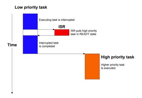
A pure cooperative multi-tasking system has the disadvantage of longer reaction times when high priority tasks become ready for execution. This makes their usage in embedded systems uncommon.
