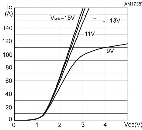
**Figure 7: Output characteristics ( $T_J = 175^\circ\text{C}$ )**
