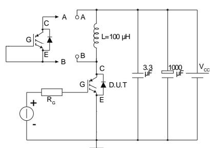
**Figure 35: Gate charge test circuit**
