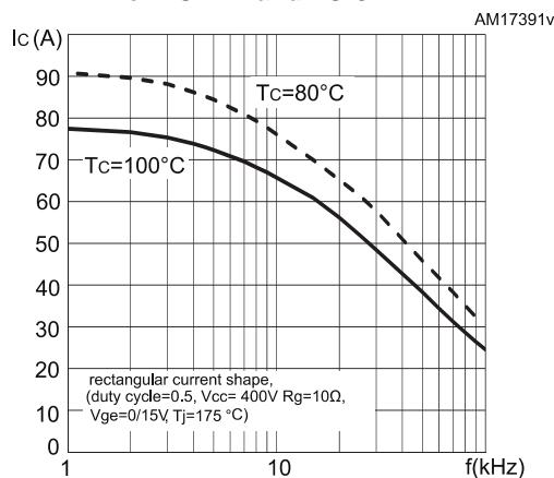
**Figure 11: Collector current vs switching frequency for TO-3PF**
