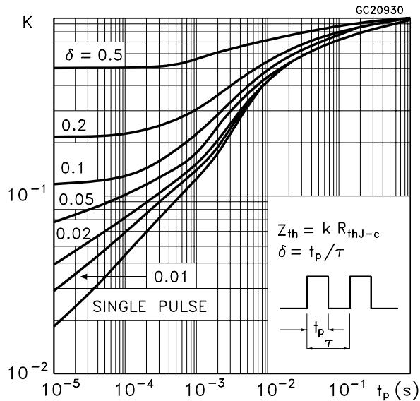
Figure 33: Thermal impedance for diode in TO-3PF
