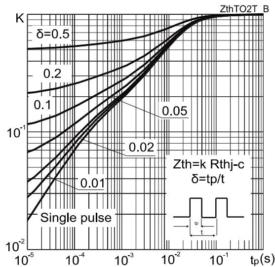
**Figure 31: Thermal impedance for IGBT in TO-3PF**
