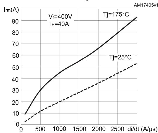
**Figure 27: Reverse recovery time vs diode current slope**
