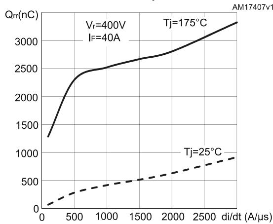
**Figure 29: Reverse recovery energy vs diode current slope**
