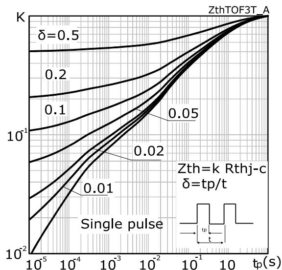
Figure 32: Thermal impedance for diode in TO-247 and TO-3P
