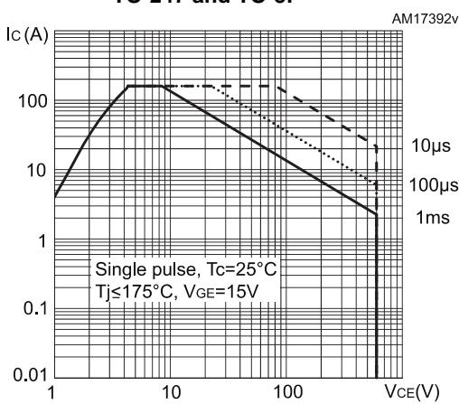
**Figure 13: Forward bias safe operating area for TO-3PF**
