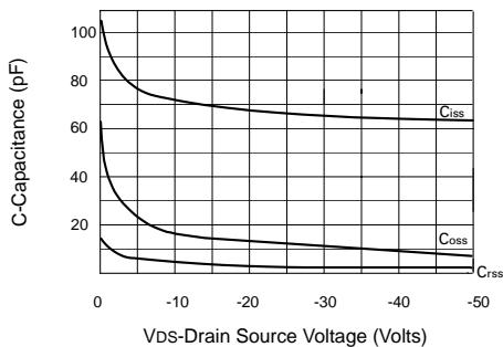
**Capacitance v drain-source voltage**
