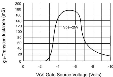
**Transconductance v gate-source voltage**
