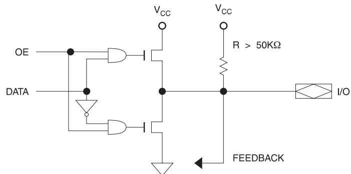
**Figure 14-3.** Functional Logic Diagram Atmel ATF22V10B
