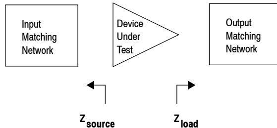
Figure 12. Series Equivalent Source and Load Impedance
