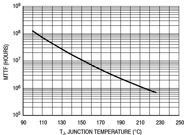
This above graph displays calculated MTTF in hours when the device is operated at  $V_{DD} = 50 \text{ Vdc}$ ,  $P_{out} = 10 \text{ W Peak}$ , Pulse Width =  $100 \mu\text{sec}$ , Duty Cycle = 20%, and  $\eta_D = 69\%$ .
