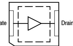
Note: The center pad on the backside of the package is the source terminal for the transistor.
