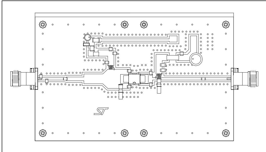
**Figure 17.** Test circuit photomaster
