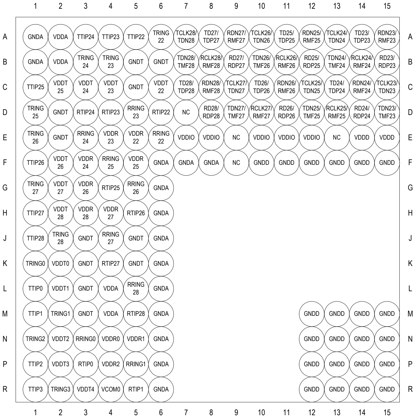
Figure-3 640-Pin PBGA (Top View) - Top Left
