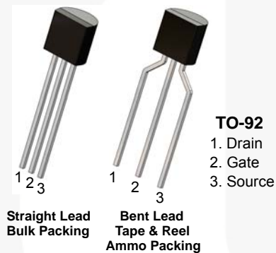
Figure 1. J175 / J176 Device Package
