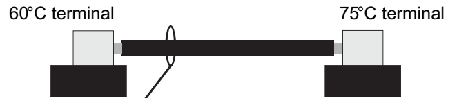
Conductor size and insulation rating?
