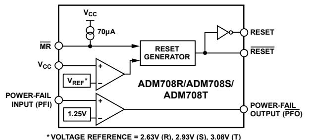
Figure 14. ADM708 Functional Block Diagram
