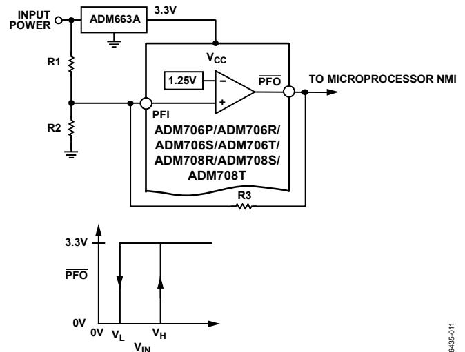
Figure 18. Adding Hysteresis to the Power-Fail Comparator
