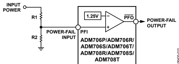
Figure 17. Power-Fail Comparator
