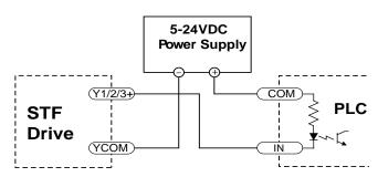
Connecting a sinking output with PLC's input
