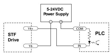
Connecting a sinking output with PLC's input
