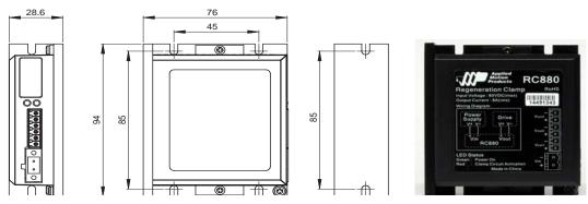
When using a regulated power supply you may encounter a problem with regeneration. The kinetic energy caused by regeneration is transferred back to the power supply. This can trip the overvoltage protection of a switching power supply, causing it to shut down. Applied Motion Products offers the RC880 "regeneration clamp" to solve this problem. If in doubt, use an RC880 for the first installation. If the "regen" LED on the RC880 never flashes, you don't need the clamp.
