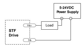
Connecting a sinking output
