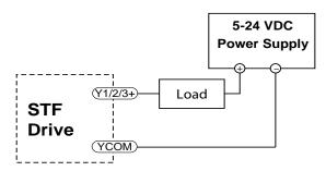
Connecting a sinking output
