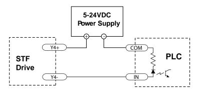
Connecting a sourcing output with PLC's input
