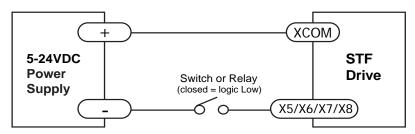
Connecting the inputs to a Switch or Relay
