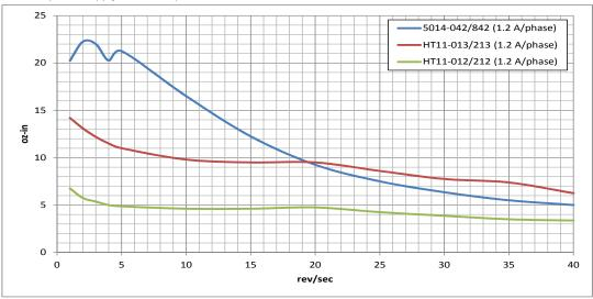
**HT17**24 VDC power supply, 20000 steps/rev, all motors connected in parallel
