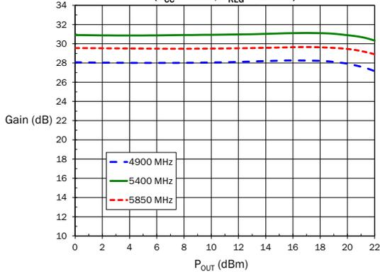
Typical Gain @ 5400MHz versus  $P_{OUT}$  over Temp (-40 to +85C)
