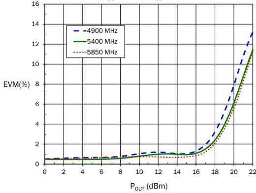
Typical EVM versus  $P_{OUT}$  over Temperature -40 TO +85C
