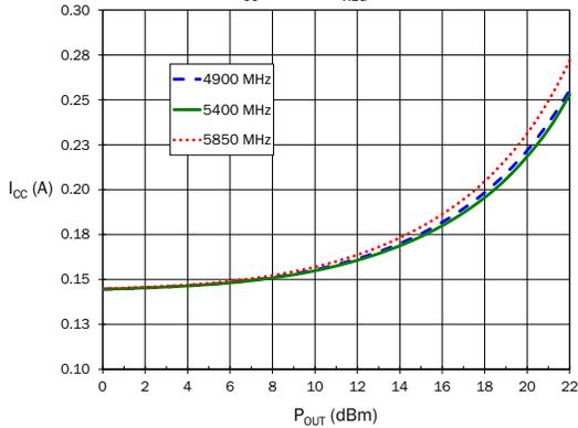
Typical  $I_{CC}$  versus  $P_{OUT}$  over Temp (-40 to +85C)
