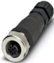
Sensor/actuator socket, straight, 4-pos., M12, A-coded, screw connection, metal knurl, cable gland Pg7 SKINTOP®
