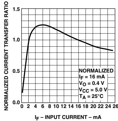
Figure 2. Current Transfer Ratio vs. Input Current.
