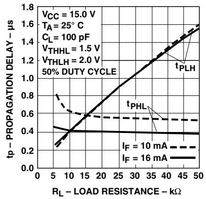
Figure 12. Propagation Delay Time vs. Load Resistance.
