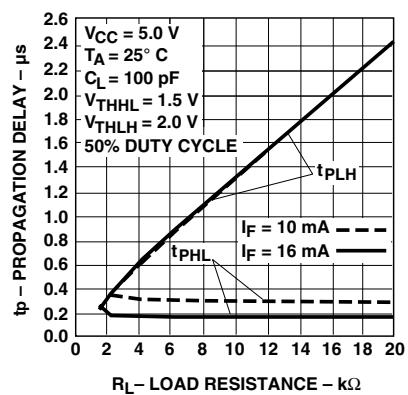
Figure 10. Propagation Delay Time vs. Load Resistance.
