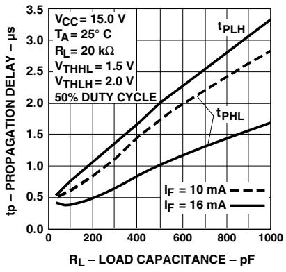
Figure 13. Propagation Delay Time vs. Load Capacitance.
