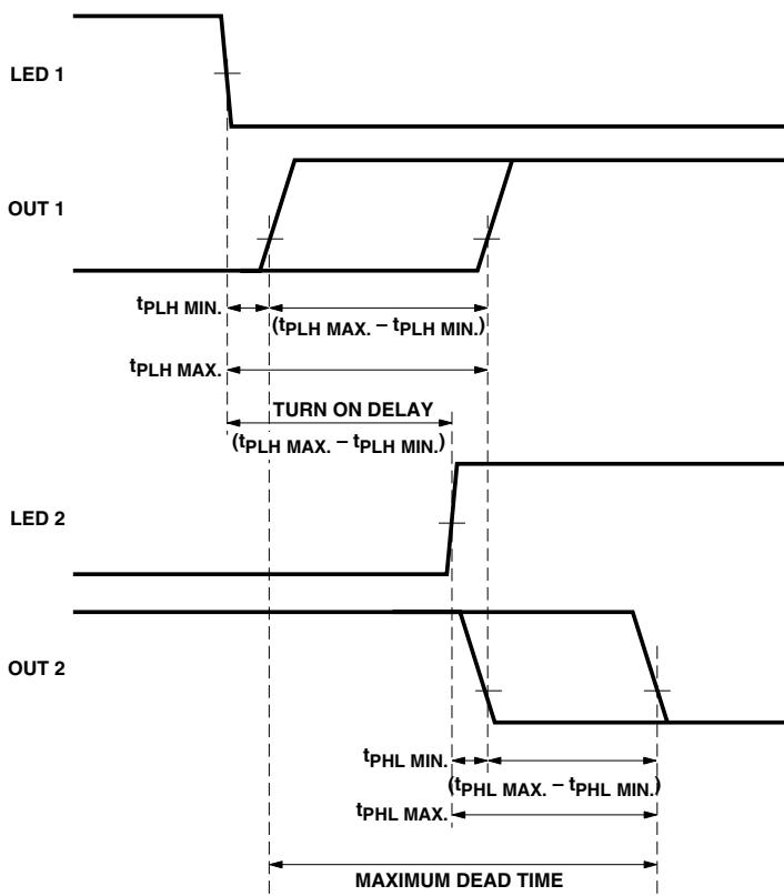
Figure 16. LED Delay and Dead Time Diagram.
