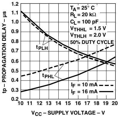
Figure 14. Propagation Delay Time vs. Supply Voltage.
