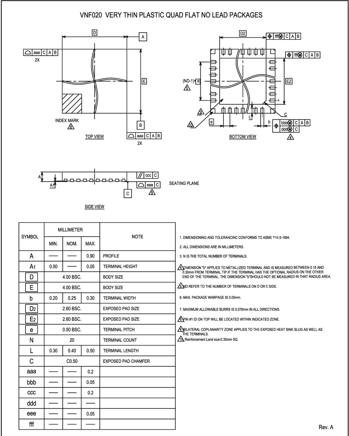
Figure 18-2 Package Dimensions of S6AE103A (VNF024)
