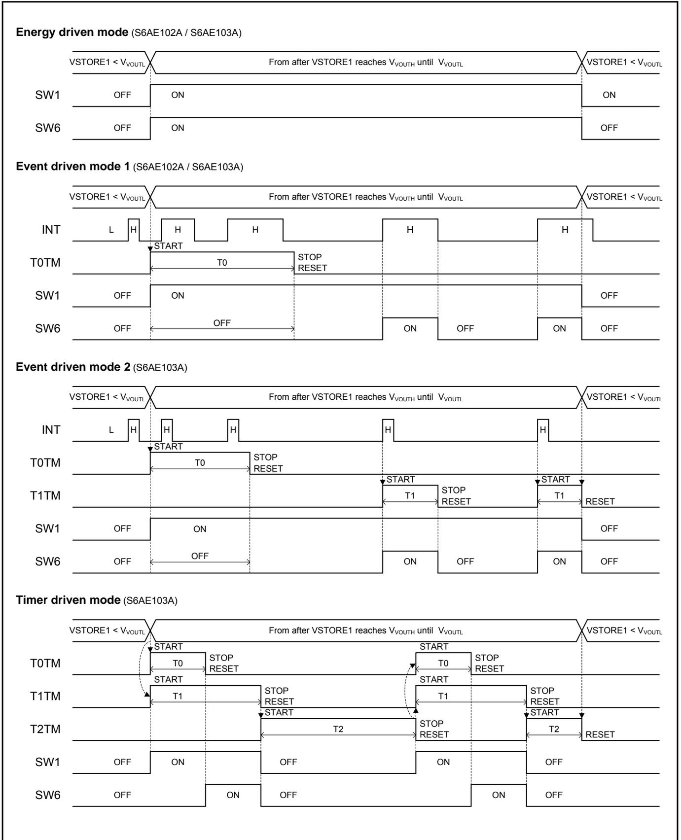
Figure 12-7 Power Gating Operation (VBAT Input Power)
