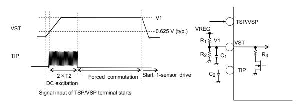
VST voltage is calculated from the following formula. (t = 0 s in startup)
