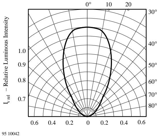
Figure 4 Rel. Luminous Intensity vs. Angular Displacement
