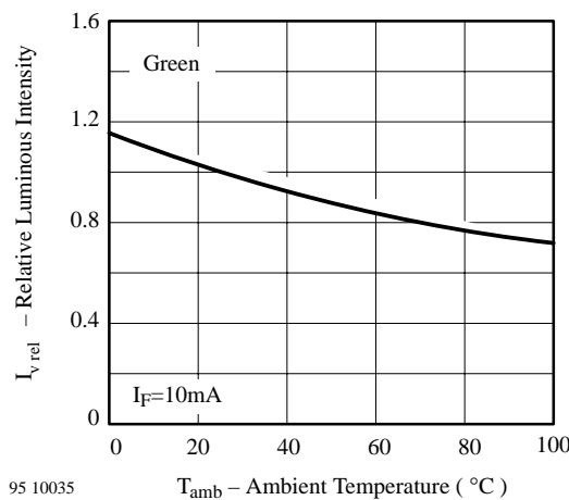
Figure 11 Rel. Luminous Intensity vs. Ambient Temperature
