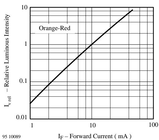
Figure 8 Relative Luminous Intensity vs. Forward Current
