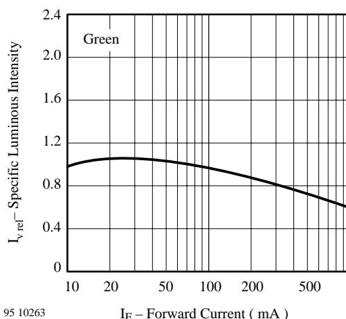
Figure 12 Specific Luminous Intensity vs. Forward Current
