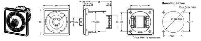
**Note:** Tightening torque for panel mounting is as follows:  $300 \text{ m N} \cdot \text{m} \pm 50 \text{ m N} \cdot \text{m}$
