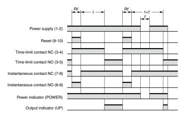
**Note:** t is the set time, Rt' is the reset application time, and t' is the power interruption time.
