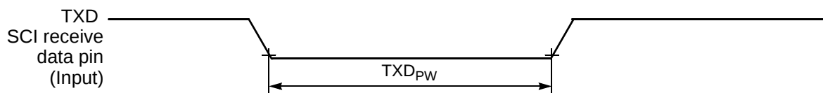
Figure 10-18 TXD Pulse Width
