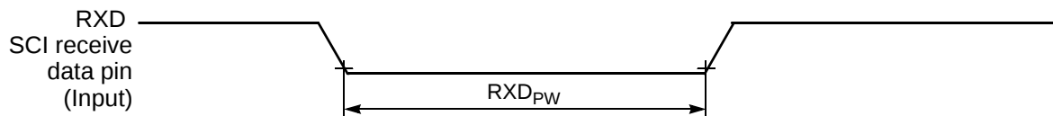
Figure 10-17 RXD Pulse Width
