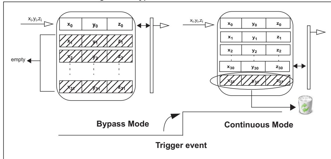
**Figure 14. Trigger event to FIFO for Bypass-to-Continuous mode**
