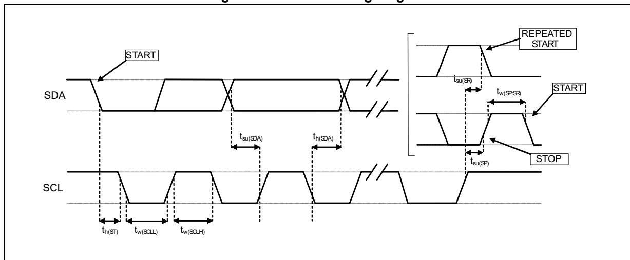
Note: Measurement points are done at 0.2·Vdd\_IO and 0.8·Vdd\_IO, for both ports.
