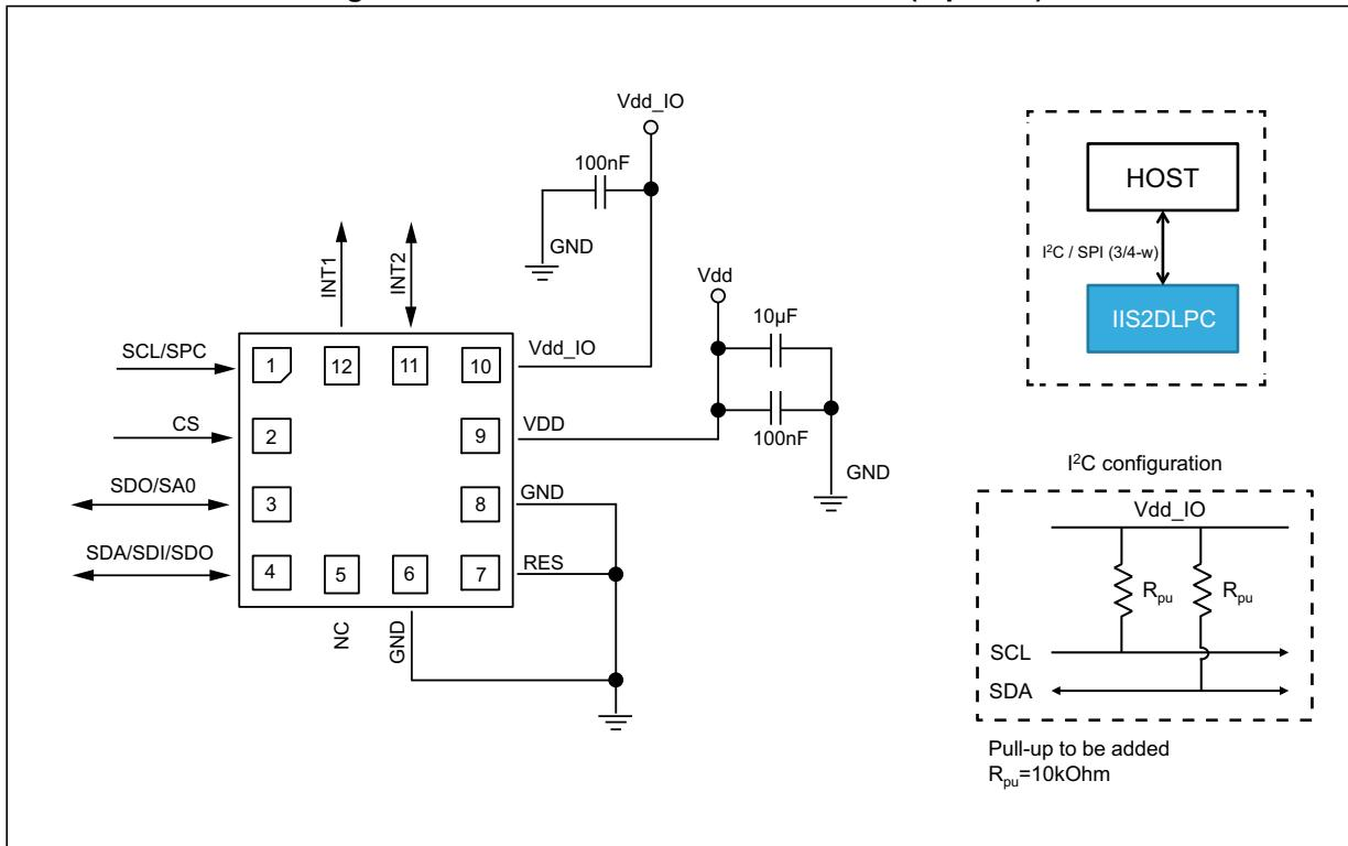
The device core is supplied through the Vdd line while the I/O pads are supplied through the Vdd\_IO line. Power supply decoupling capacitors (100 nF ceramic, 10 µF aluminum) should be placed as near as possible to pin 9 of the device (common design practice).
