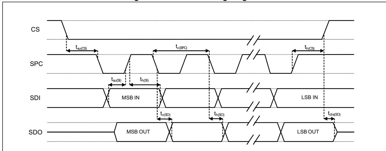
*Measurement points are done at  $0.2 \cdot Vdd\_IO$  and  $0.8 \cdot Vdd\_IO$ , for both input and output ports.*
