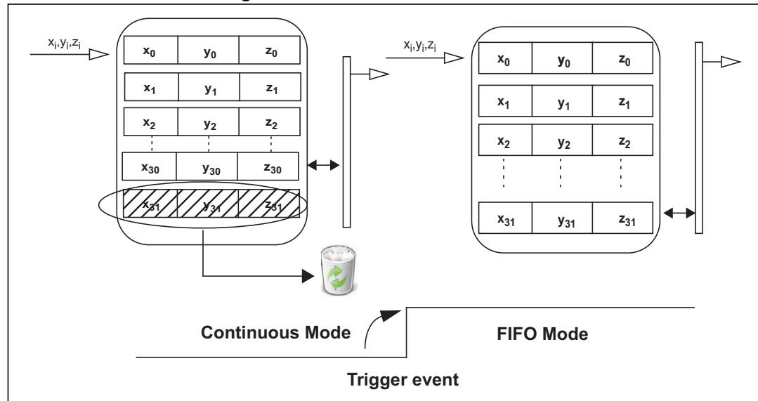
Figure 12. Trigger event to FIFO for Continuous-to-FIFO mode
