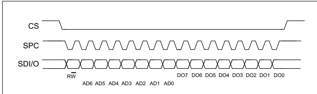
The SPI read command is performed with 16 clock pulses:
