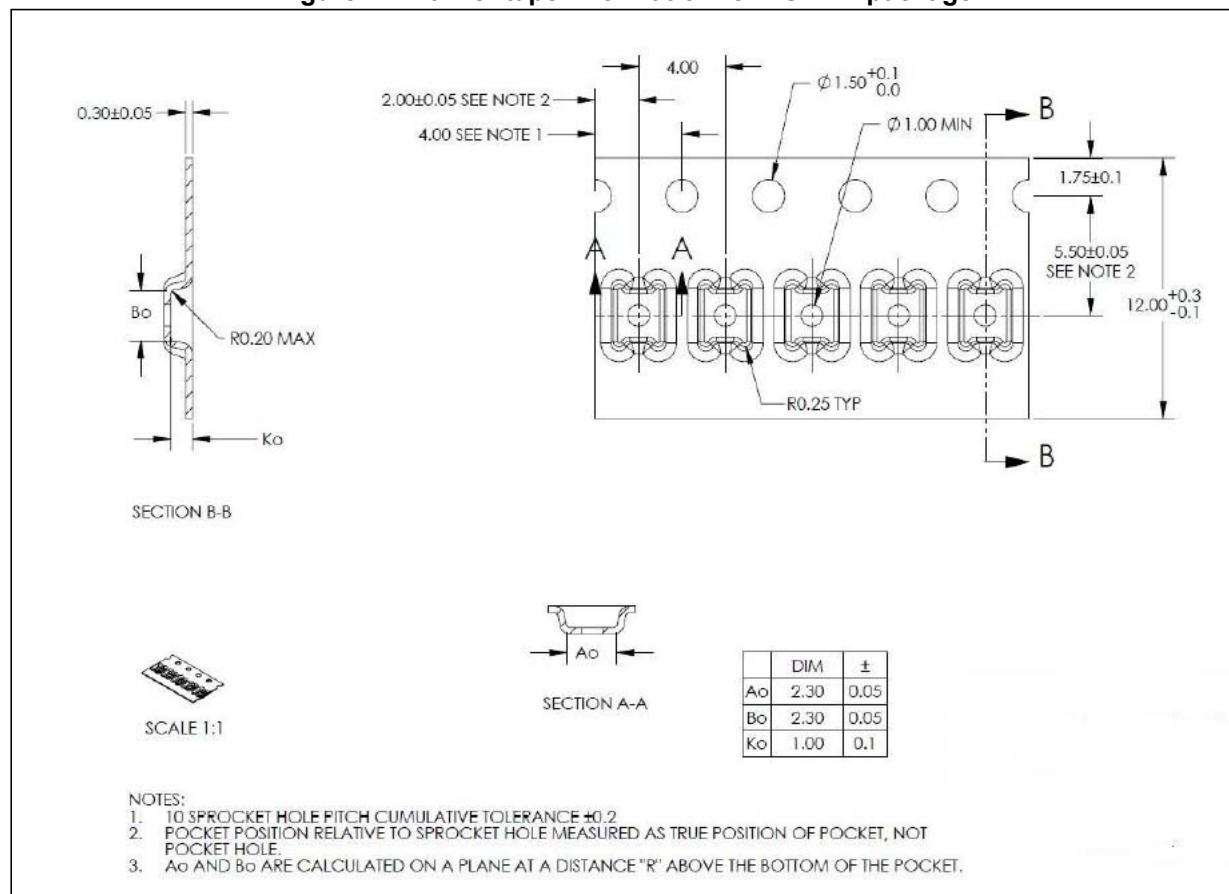
Figure 23. LGA-12 package orientation in carrier tape
