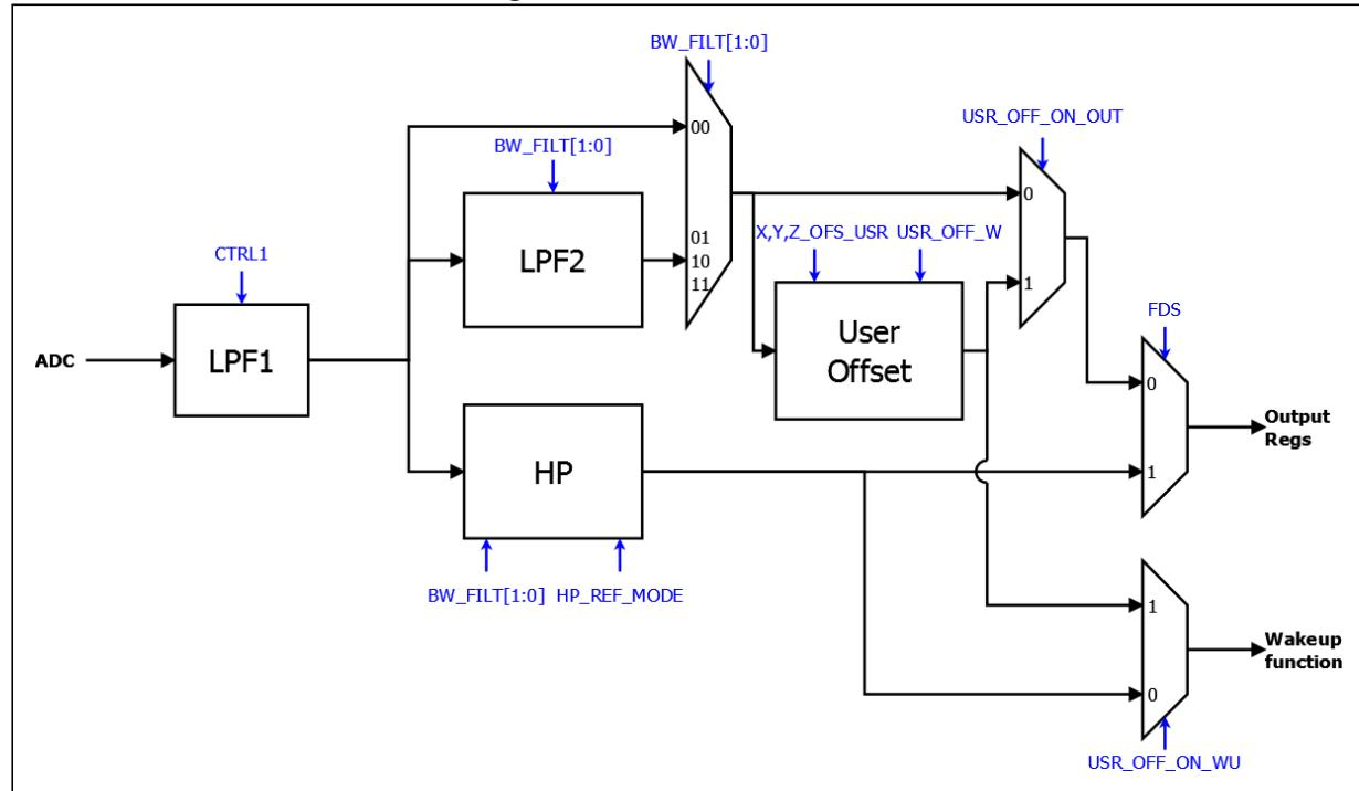
Referring to [Figure 7](#), the first block is the Low-Pass Filter 1 (LPF1) whose behavior is a function of the actual ODR and mode selected in [CTRL1 \(20h\)](#). The signal is then downsampled and can be either directly sent to the output registers or to the Low-Pass Filter 2 (LPF2) or High-Pass-Filter (HP) using the BW\_FILT[1:0] bits and FDS bit in [CTRL6 \(25h\)](#).
