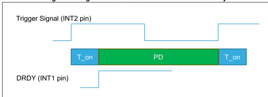
At the end of turn-on time  $T_{on}$ , the DRDY interrupt is activated, output data are available to be read and the device goes into power-down.  $T_{on}$  values depend on the low-power mode as follows:
