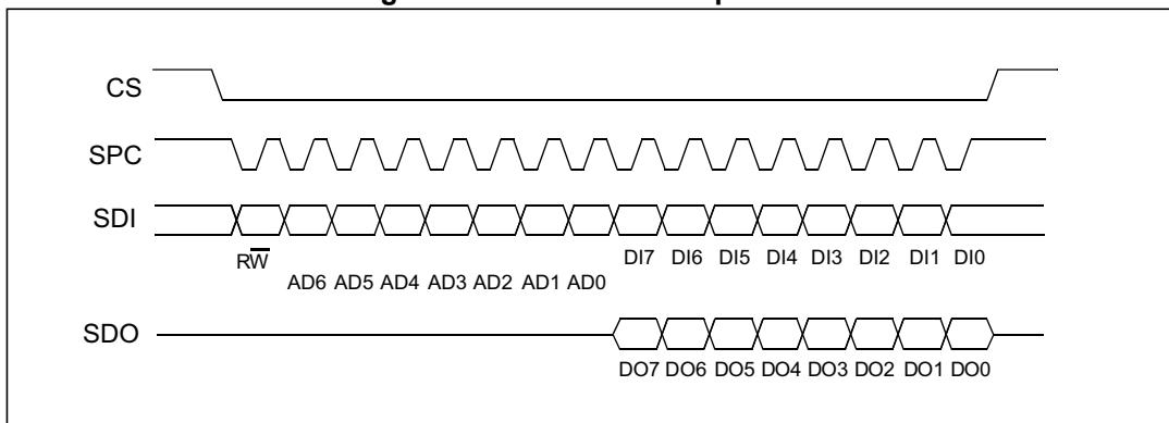
**CS** is the serial port enable and it is controlled by the SPI master. It goes low at the start of the transmission and goes back high at the end. **SPC** is the serial port clock and it is controlled by the SPI master. It is stopped high when **CS** is high (no transmission). **SDI** and **SDO** are respectively the serial port data input and output. Those lines are driven at the falling edge of **SPC** and should be captured at the rising edge of **SPC**.
