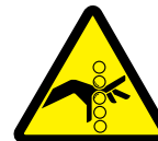
W3153 Pinch Point Hazard
