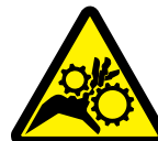
W3156 Gear Entanglement Hazard
