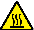
W3198 Heated/Hot Surface Hazard
