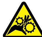
W3156 Gear Entanglement Hazard
