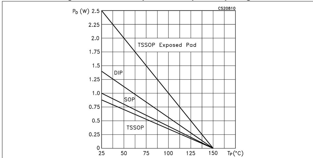
Note: The exposed-pad should be soldered to the PBC to realize the thermal benefits.
