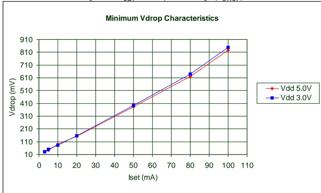
Table 11. I<sub>SET</sub> vs drop out voltage (V<sub>DROP</sub>)
