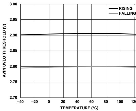
Figure 8. AVIN UVLO Threshold vs. Temperature
