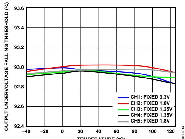
Figure 14. Output Undervoltage Falling Threshold vs. Temperature
