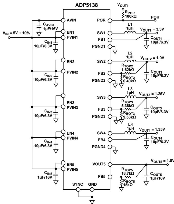
Figure 48. Application Circuit
