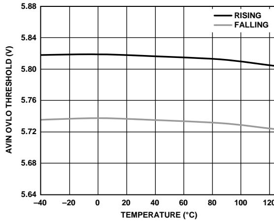
Figure 9. AVIN OVLO Threshold vs. Temperature
