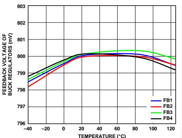
Figure 12. Feedback Voltage of Buck Regulators vs. Temperature
