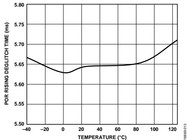
Figure 13. POR Rising Deglitch Time vs. Temperature
