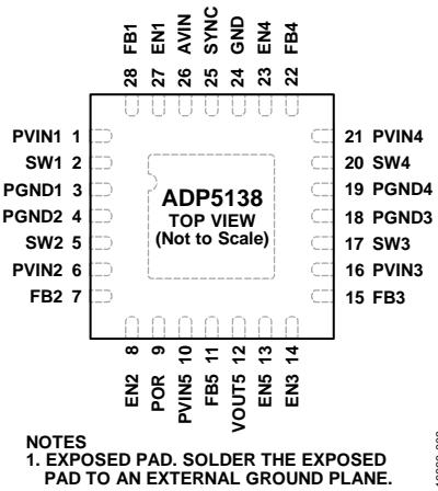
Figure 3. Pin Configuration
