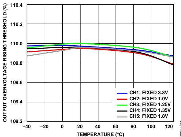
Figure 11. Output Overvoltage Rising Threshold vs. Temperature
