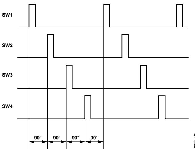
Figure 45. Even Phase Shift Between Channel 1 and Channel 4
