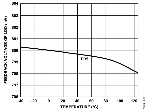
Figure 15. Feedback Voltage of LDO vs. Temperature
