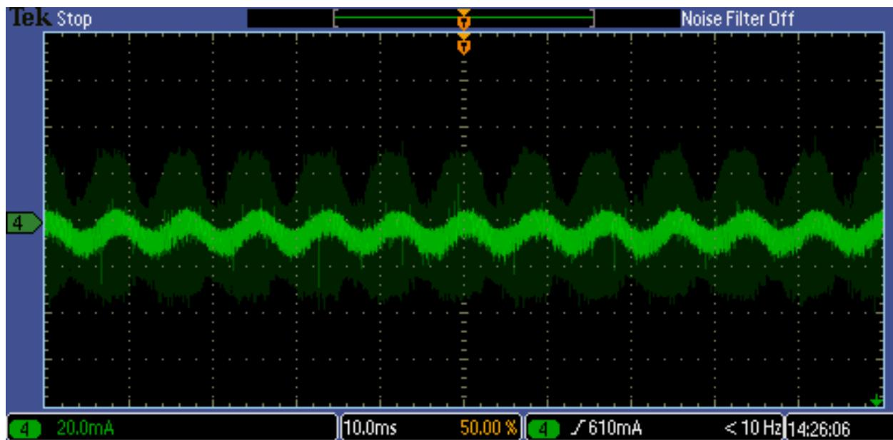
Figure 24. Ripple Current at 120 V ac Maximum Load
