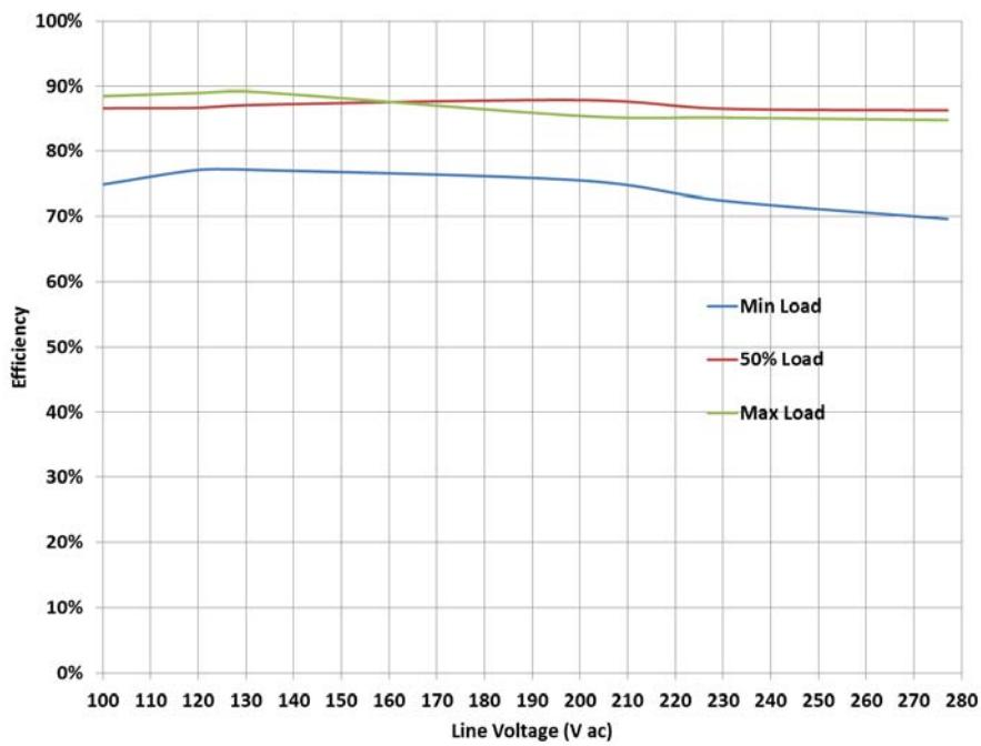
Figure 19. Efficiency over Line and Load @ 60 V dc Output
