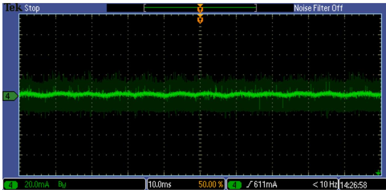
Figure 25. Ripple Current at 277 V ac Maximum Load
