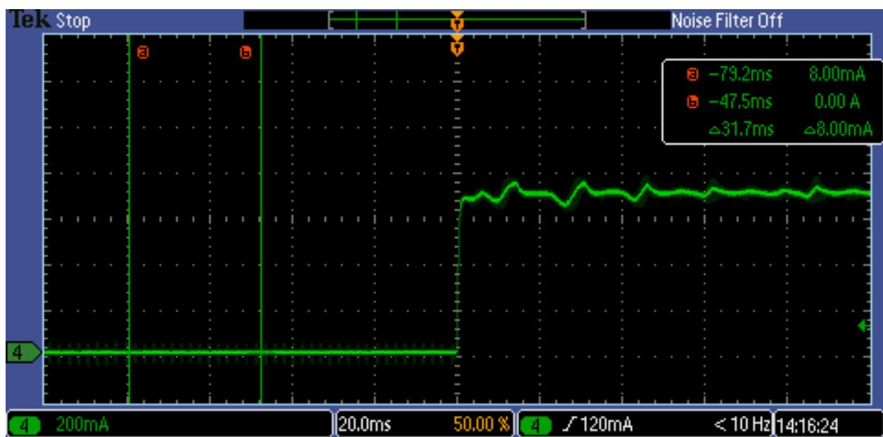
Figure 27. Start Up with On/Off 120 V Maximum Load
