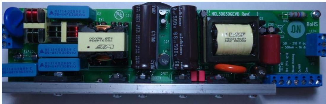
**Figure 1. Evaluation Board Picture (Top View)**
