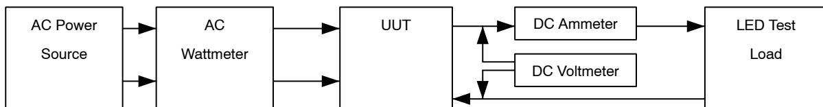
NOTE: Unless otherwise specified, all voltage measurements are taken at the terminals of the UUT.
