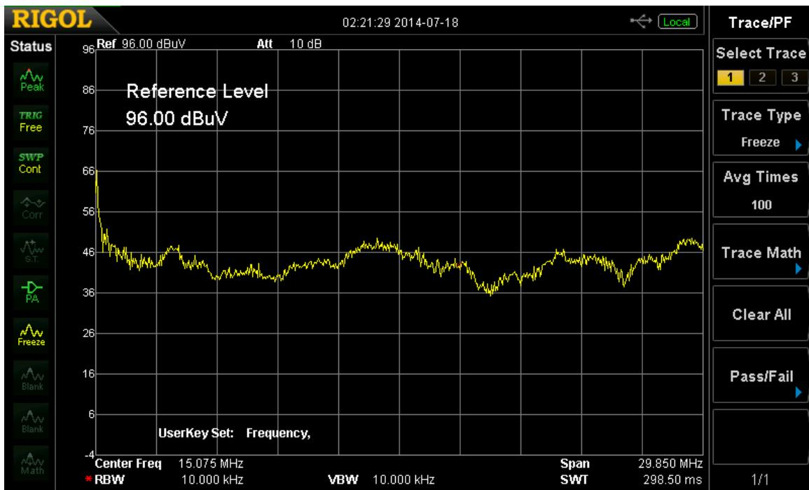
Figure 31. Conducted EMI Pre-compliance Peak Data 150 kHz – 30 MHz
