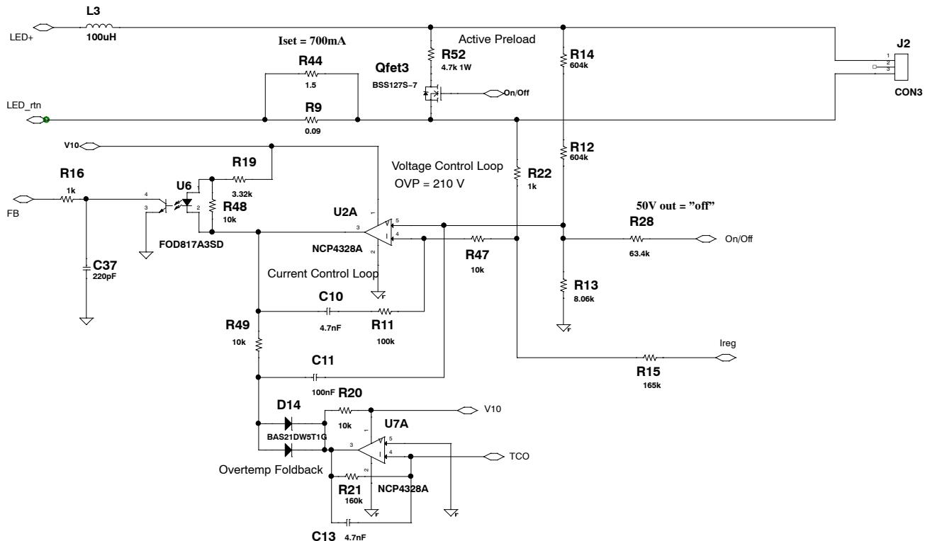
Figure 7. Control Schematic
