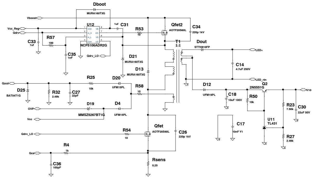
Figure 6. Flyback Schematic
