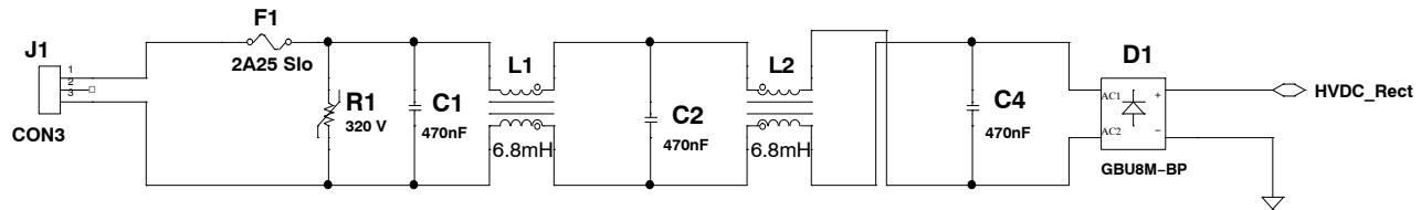
Figure 4. Input Circuit
