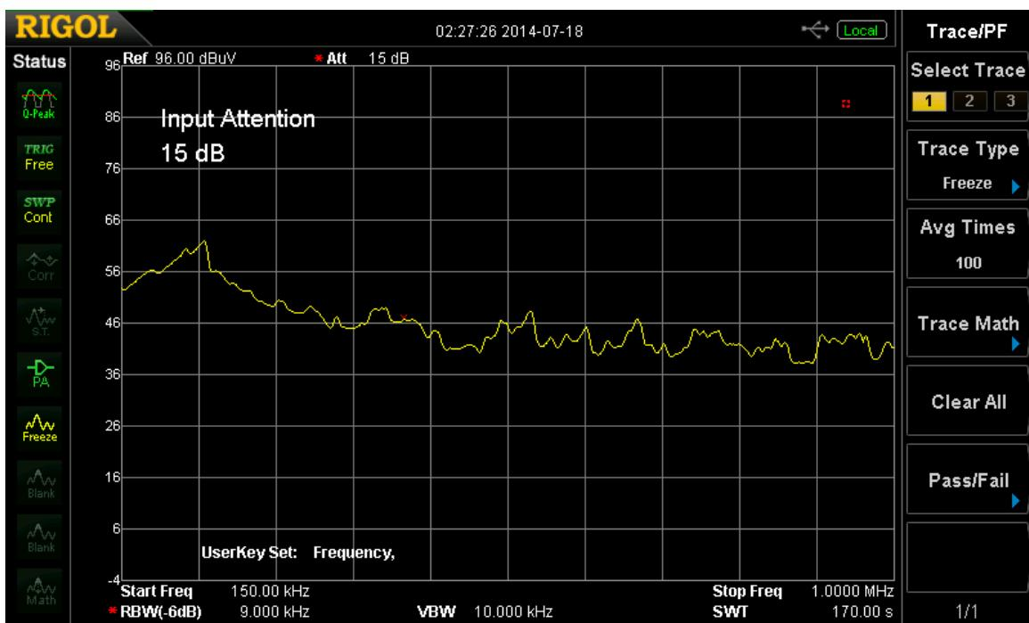
Figure 30. Conducted EMI Pre-compliance QP Data 150 kHz – 1 MHz
