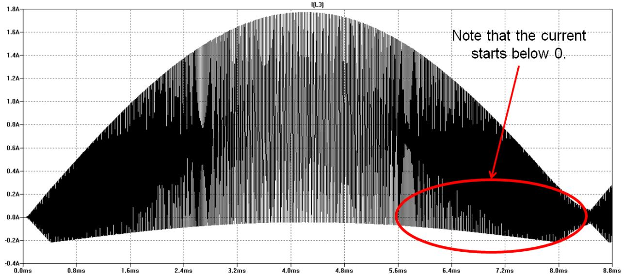
**Figure 2. Inductor Current across a Line Cycle**
