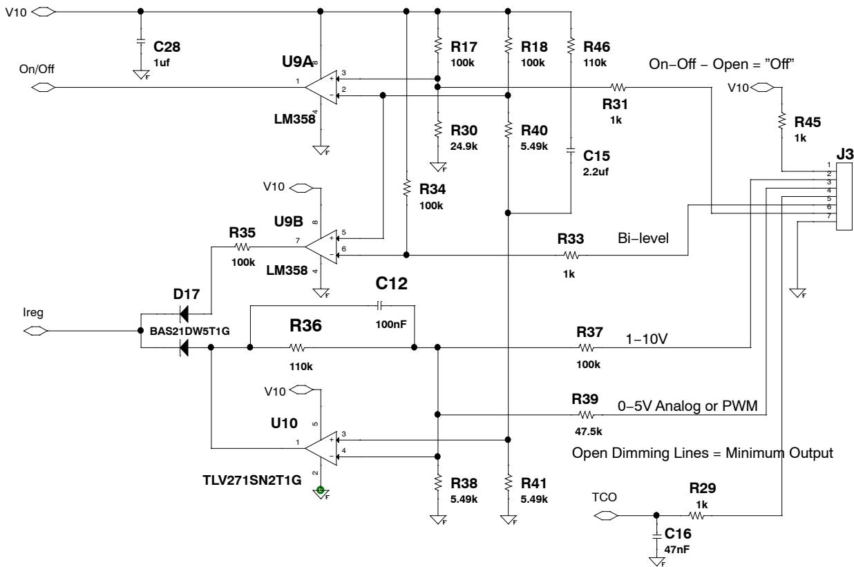
**Figure 8. Dimming Interface**
