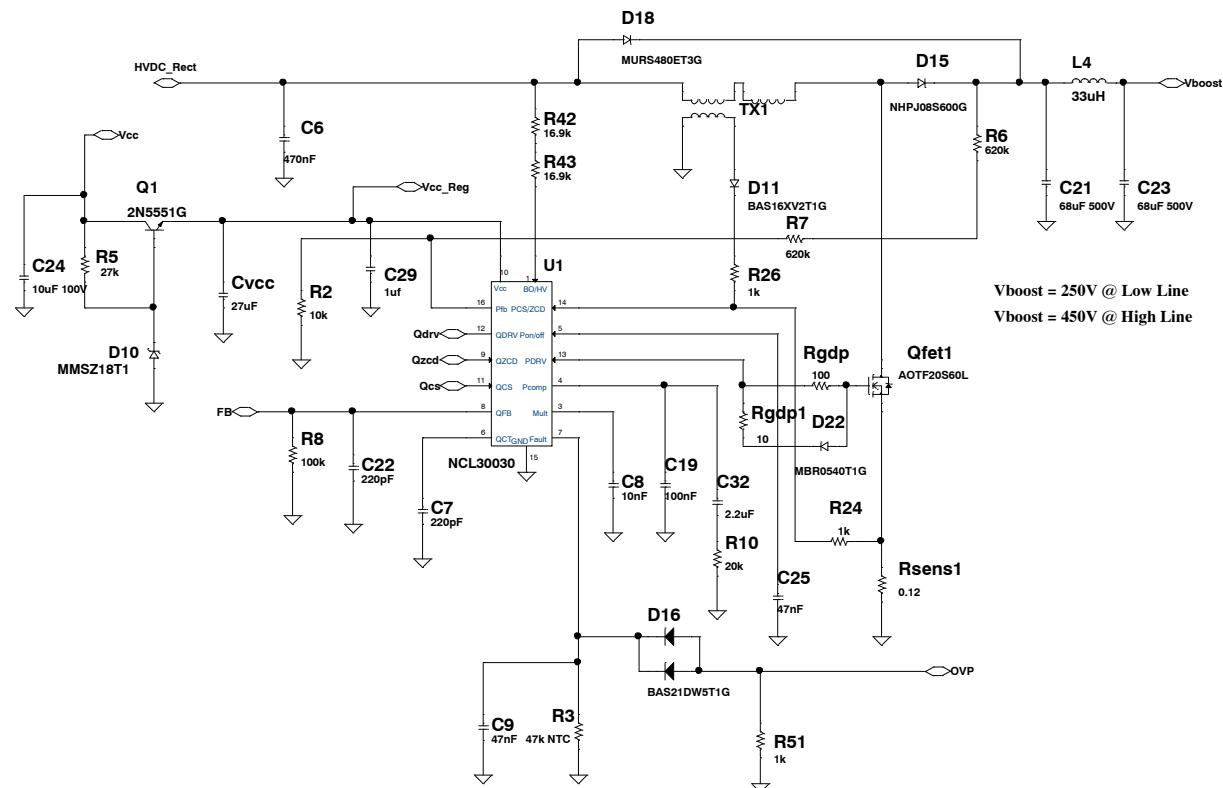
Figure 5. PFC Schematic
