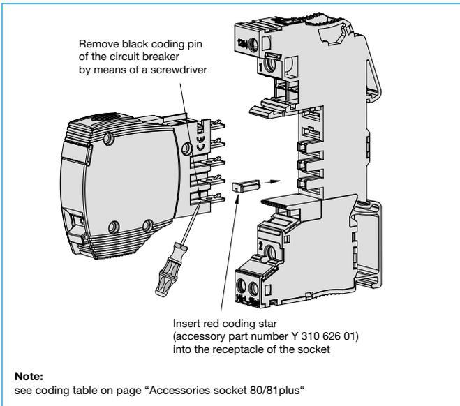
**Replacing a circuit breaker**
