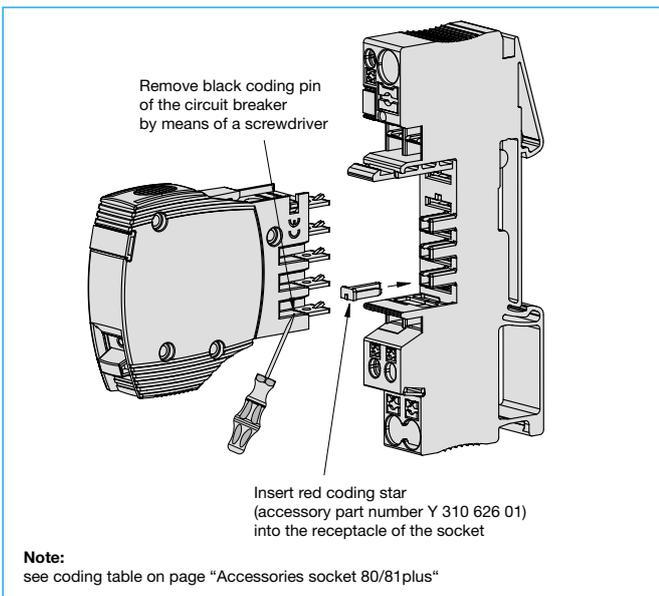
**Replacing a circuit breaker**
