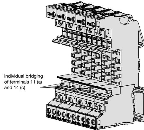
**Parallel connection of auxiliary contacts**
