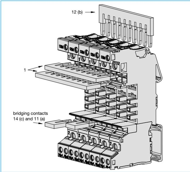
**Coding of circuit breaker 2216-S and socket 81plus following the lock-key-principle**
