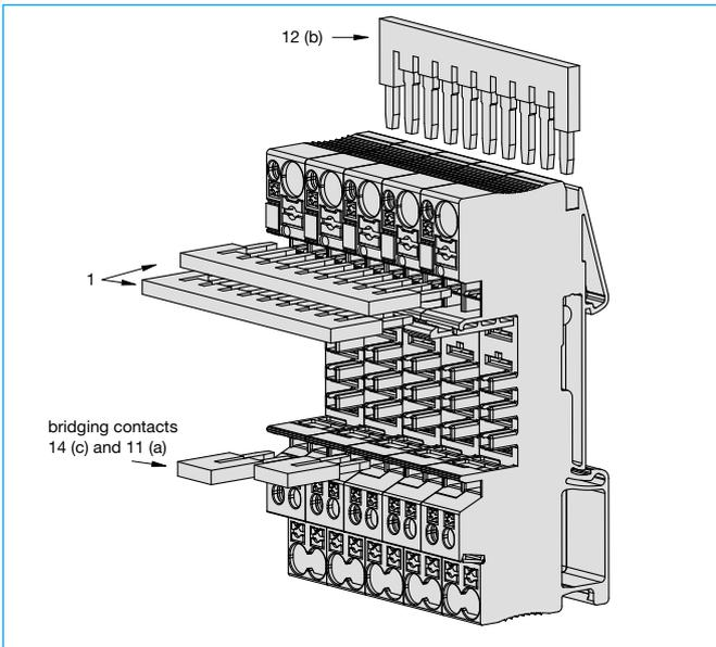
**Coding of circuit breaker 2216-S and socket 80plus following the lock-key-principle**
