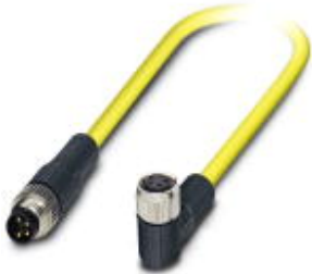
Sensor/Actuator cable, 4-position, PVC, Yellow RAL 1021, Plug straight M8, on Socket angled M8, Cable length: 0.5 m
