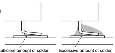
Check the soldering in the actual mounting conditions before use.
