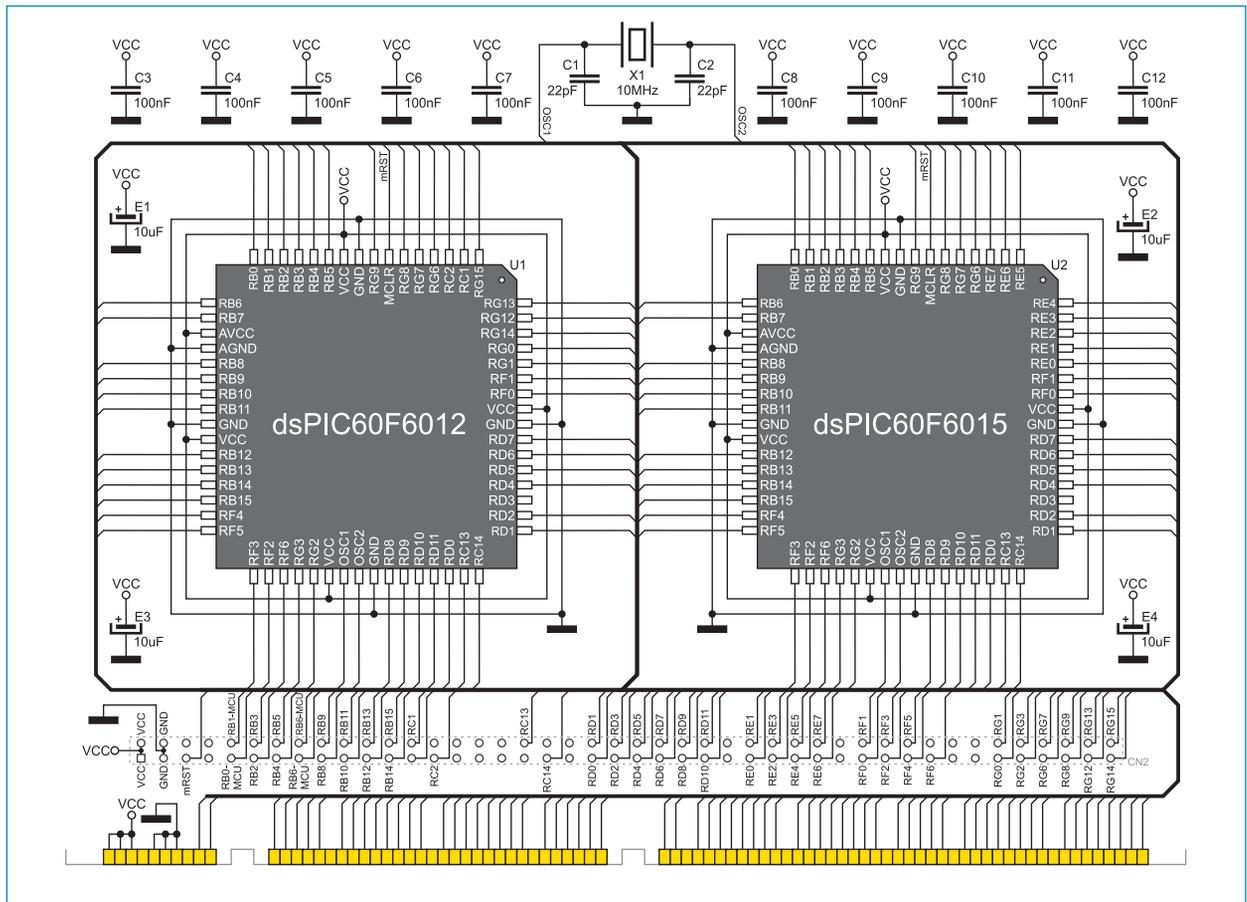
Figure 1: 64-pin MCU card and microcontroller connection schematic
