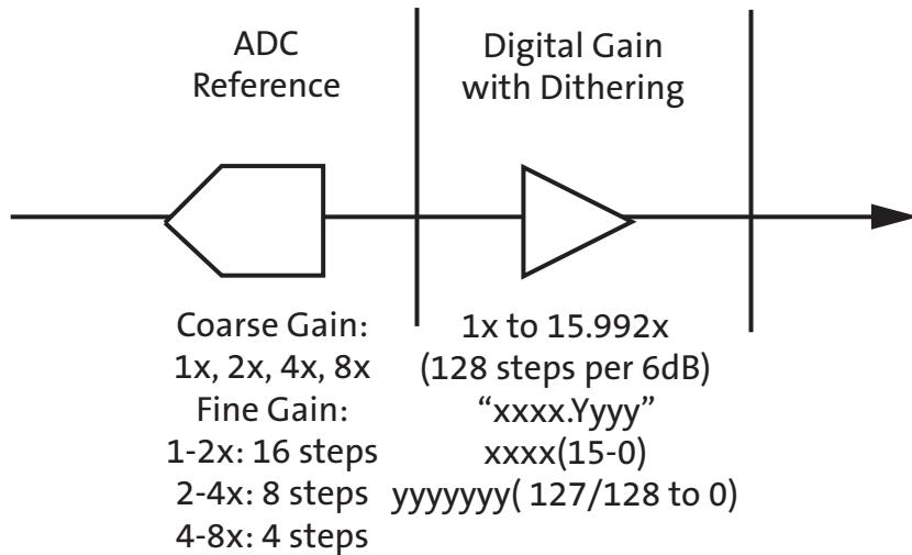
The level of analog gain applied is controlled by the coarse\_gain and fine\_gain registers. The analog readout can be configured differently for each gain level. The recommended gain tables are listed in Table 32. It is recommended that these registers are configured before streaming images.
