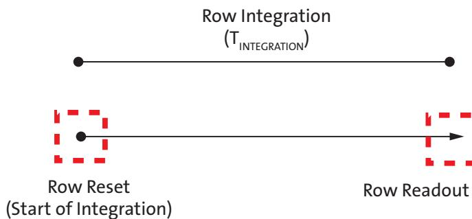
A pixel's integration time is defined by the number of clock periods between a row's reset and read operation. Both the read followed by the reset operations occur within a row period ( $T_{ROW}$ ) where the read and reset may be applied to different rows. The read and reset operations will be applied to the rows of the pixel array in a consecutive order.
