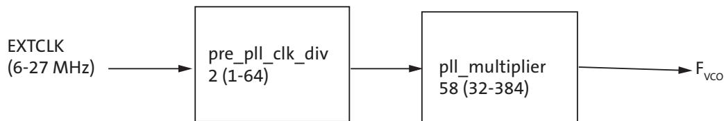
The sensor contains a phase-locked loop (PLL) that is used for timing generation and control. The required VCO clock frequency is attained through the use of a pre-PLL clock divider followed by a multiplier. The multiplier is followed by set of dividers used to generate the output clocks required for the sensor array, the pixel analog and digital readout paths, and the output parallel and serial interfaces.
