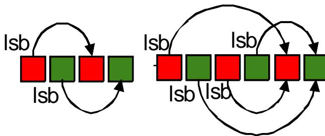
Horizontal binning is achieved either in the pixel readout or the digital readout. The sensor will sample the combined 2x or 3x adjacent pixels within the same color plane.
