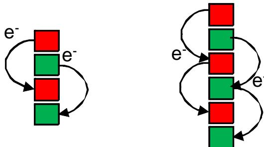
Vertical row binning is applied in the pixel readout. Row binning can be configured of 2x or 3x rows within the same color plane. ON Semiconductor recommends not to use 3x binning in AR0330 as it may introduce some image artifacts.
