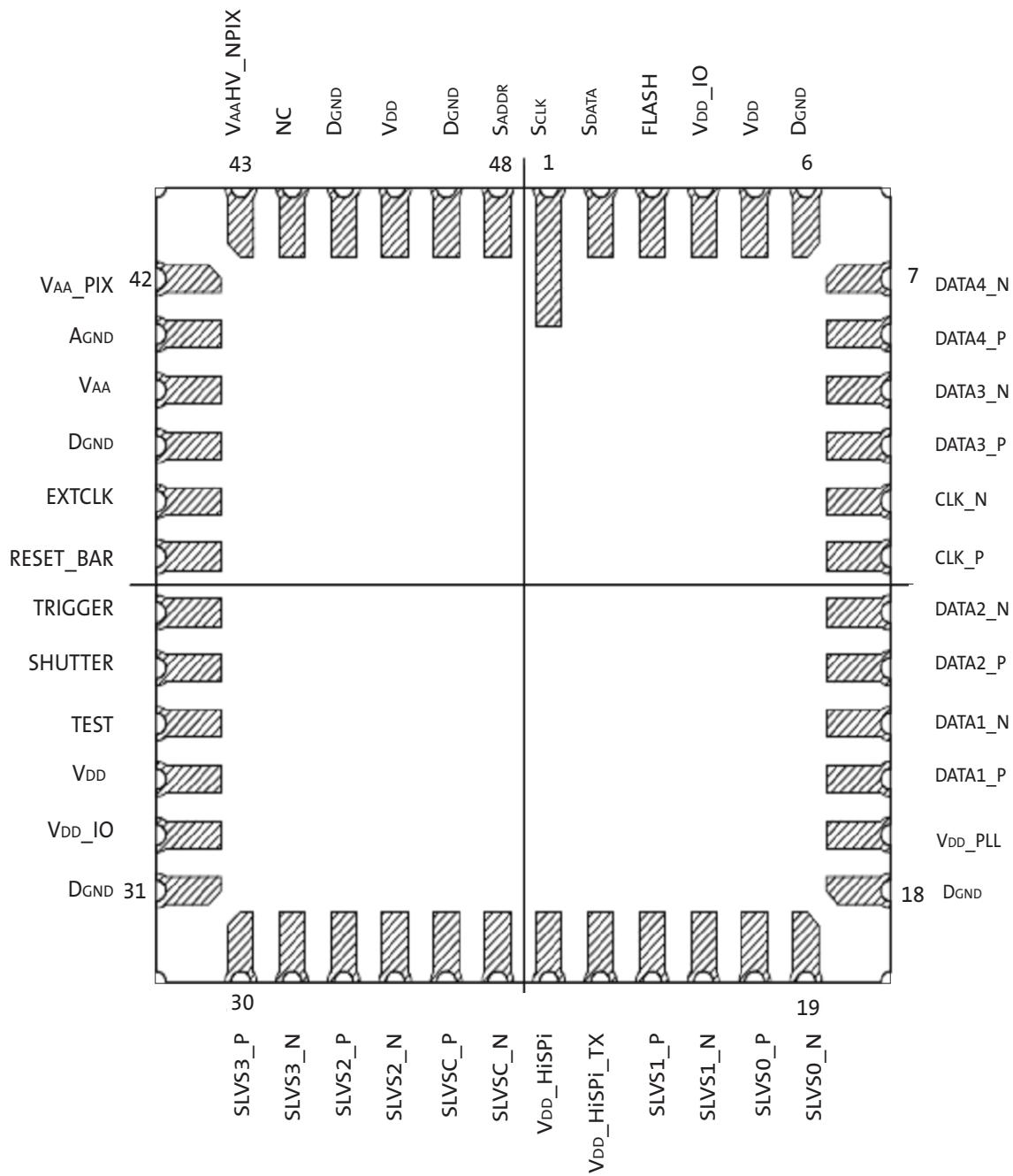
Note: Pins labeled NC (Not Connected) should be tied to ground
