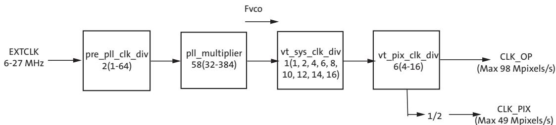
The maximum output of the parallel interface is 98 Mpixel/s (CLK\_OP). This will limit the readout clock (CLK\_PIX) to 49 Mpixel/s. The sensor will not use the  $F_{SERIAL}$ ,  $F_{SERIAL\_CLK}$  or CLK\_OP when configured to use the parallel interface.
