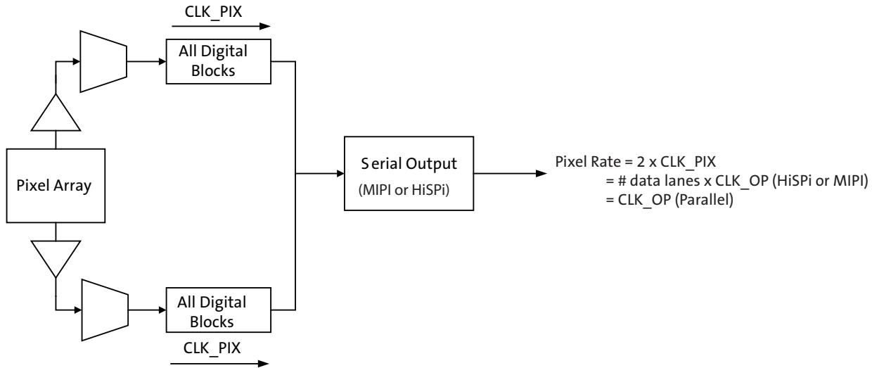
The sensor row timing calculations refers to each data-path individually. For example, the sensor default configuration uses 1248 clocks per row (`line_length_pck`) to output 2304 active pixels per row. The aggregate clocks per row seen by the receiver will be 2496 clocks (1248 x 2 readout paths).
