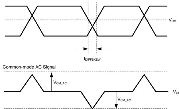
Figure 13 on page 29 also shows the corresponding AC  $V_{CM}$  common-mode signal. Differential skew between the  $V_{oa}$  and  $V_{ob}$  signals can cause spikes in the common-mode, which the receiver needs to be able to reject.  $V_{CM\_AC}$  is measured as the absolute peak deviation from the mean DC  $V_{CM}$  common-mode.
