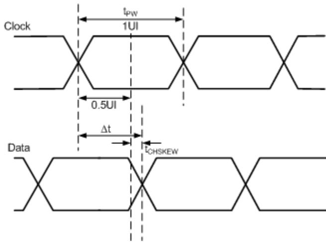
$$t_{CHSKEW}(\text{ps}) = \Delta t - \frac{t_{pw}}{2} \quad (\text{EQ } 7)$$
