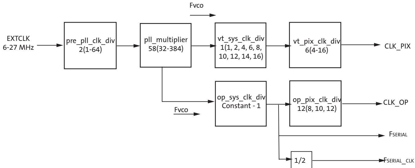
The sensor will use op<sub>\_sys</sub>\_clk<sub>\_div</sub> and op<sub>\_pix</sub>\_clk<sub>\_div</sub> to configure the output clock per lane (CLK<sub>\_OP</sub>). The configuration will depend on the number of active lanes (1, 2, or 4) configured. To configure the sensor protocol and number of lanes, refer to “Serial Configuration” on page 40.
