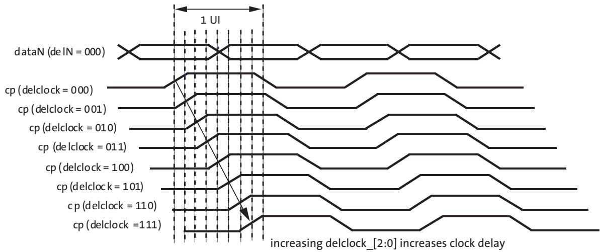
**Figure 25: Delaying data\_lane with Respect to the clock\_lane**
