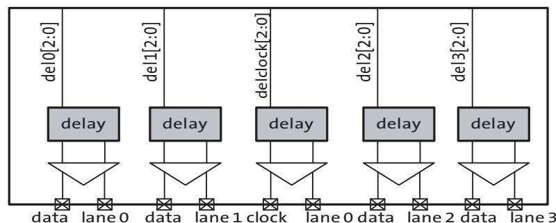
**Figure 24: Delaying the clock\_lane with Respect to data\_lane**
