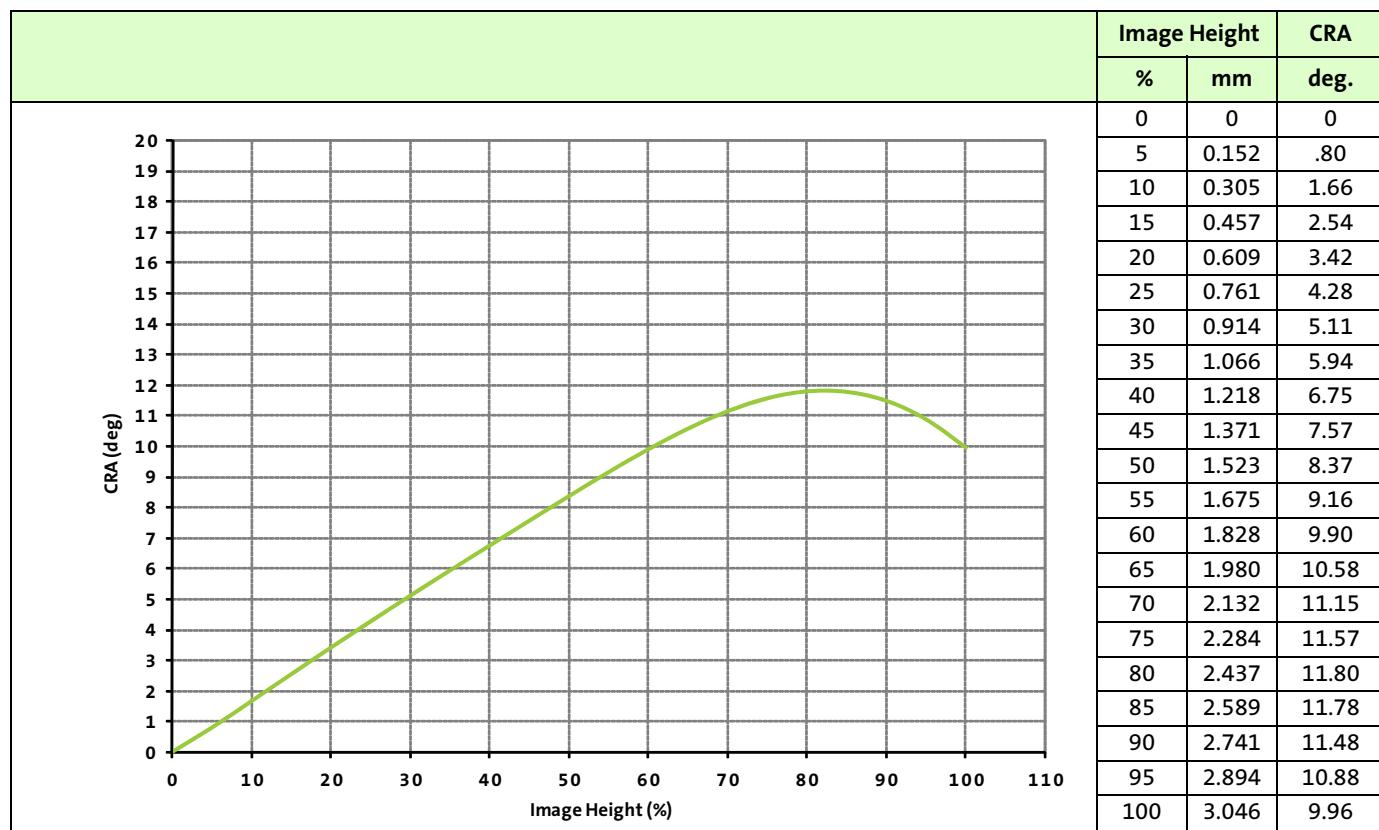
Note: The CRA listed in the advanced data sheet described the 2048x1536 field of view (2.908mm image height). This information was sufficient for configuring the sensor to read both the 4:3 (2048x1536) and 16:9 (2304x1296) aspect ratios. The CRA information listed in the data sheet has now been updated to represent the entire pixel array (2304x1536).
