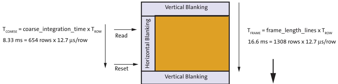
The fine integration is then defined by the number of pixel clock periods between the row reset and row read operation within  $T_{ROW}$ . This period is defined by the *fine\_integration\_time* register.
