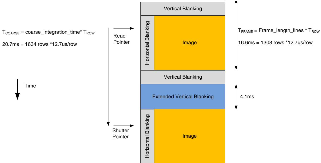
The minimum frame-time is defined by the number of row periods per frame and the row period. The sensor frame-time will increase if the *coarse\_integration\_time* is set to a value equal to or greater than the *frame\_length\_lines*. The maximum integration time can be limited to the frame time by setting R0x30CE[5] to 1.
