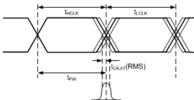
Period Jitter ( $t_{CKJIT}$ ) is defined as the deviation of the instantaneous clock  $t_{pw}$  from an ideal 1UI. This should be measured for both the clock high period variation  $\Delta t_{HCLK}$ , and the clock low period variation  $\Delta t_{LCLK}$  taking the RMS or 1-sigma standard deviation and quoting the worse case jitter between  $\Delta t_{HCLK}$  and  $\Delta t_{LCLK}$ .
