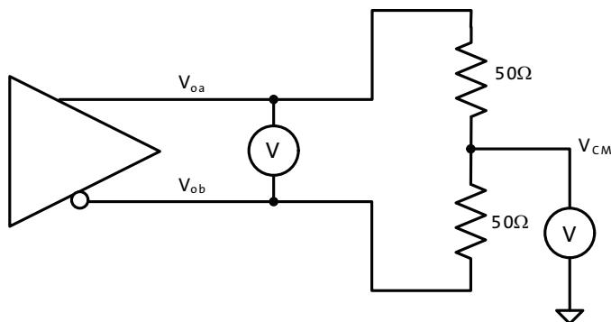
$$V_{OD}(m) = |V_{oa}(m) - V_{ob}(m)| \text{ where 'm' is either "1" for logic 1 or "0" for logic 0} \quad (\text{EQ } 1)$$
