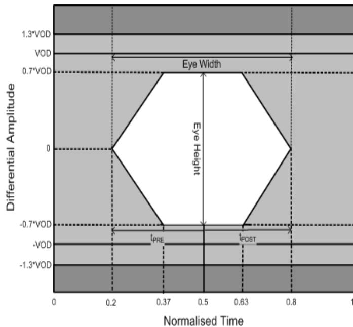
Figure 14 defines the eye mask for the transmitter. 0.5 UI point is the instantaneous crossing point of the Clock. The area in white shows the area Data is prohibited from crossing into. The eye mask also defines the minimum eye height, the data  $t_{pre}$  and  $t_{post}$  times, and the total jitter pk-pk + mean skew ( $t_{TJSKEW}$ ) for Data.
