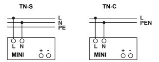
The 100...240 V AC connection is made using the L and N screw connections.
