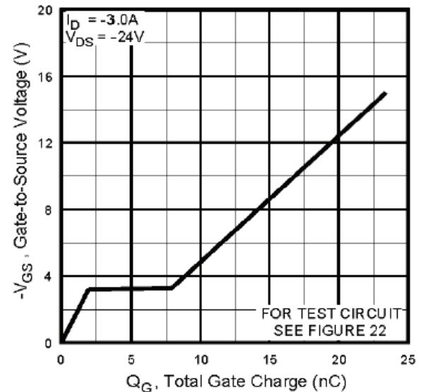
**Fig. 17.** Typical Gate Charge vs.
