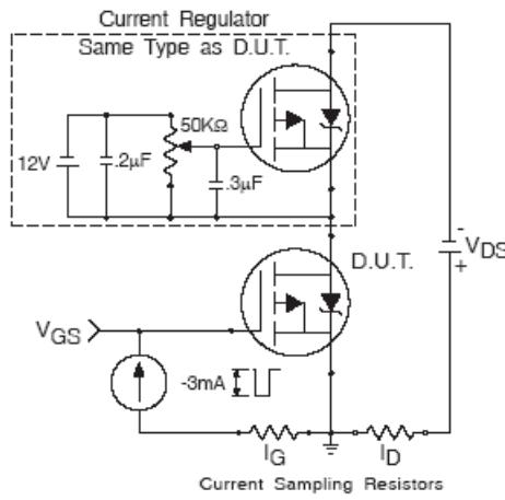
**Fig 22a.** Gate Charge Test Circuit
