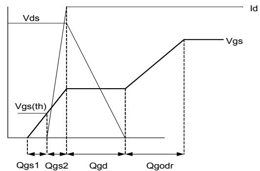
**Fig 11b.** Basic Gate Charge Waveform
