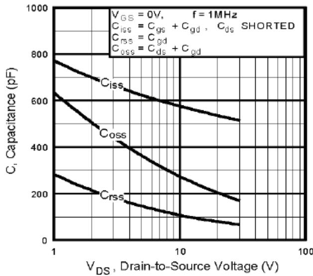
**Fig 5.** Typical Capacitance vs.
