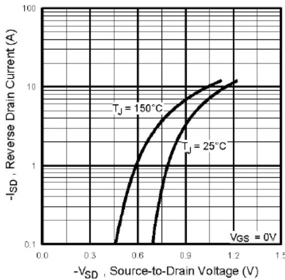
**Fig. 18** Typical Source-to-Drain Diode
