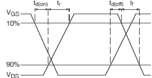
**Fig 21b.** Switching Time Waveforms
