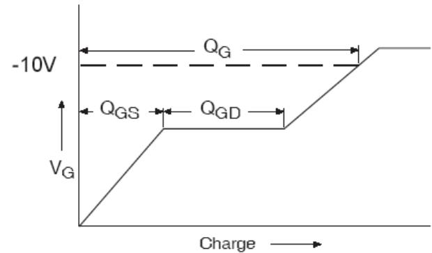
**Fig 22b.** Basic Gate Charge Waveform
