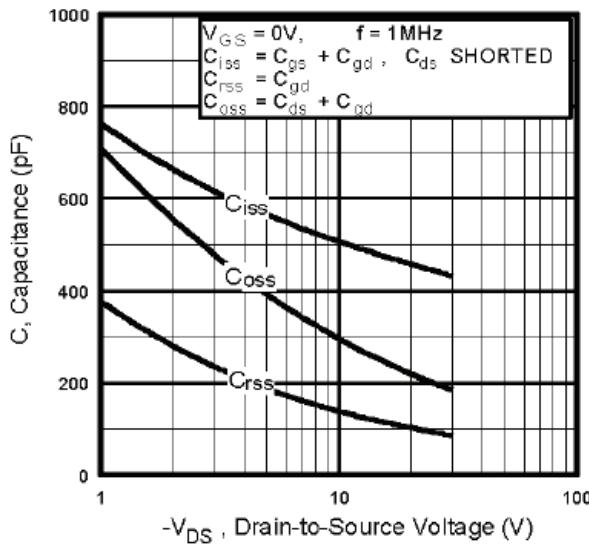
**Fig. 16.** Typical Capacitance vs.
