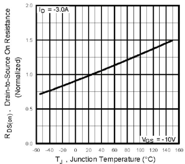
**Fig. 15** Normalized On-Resistance
