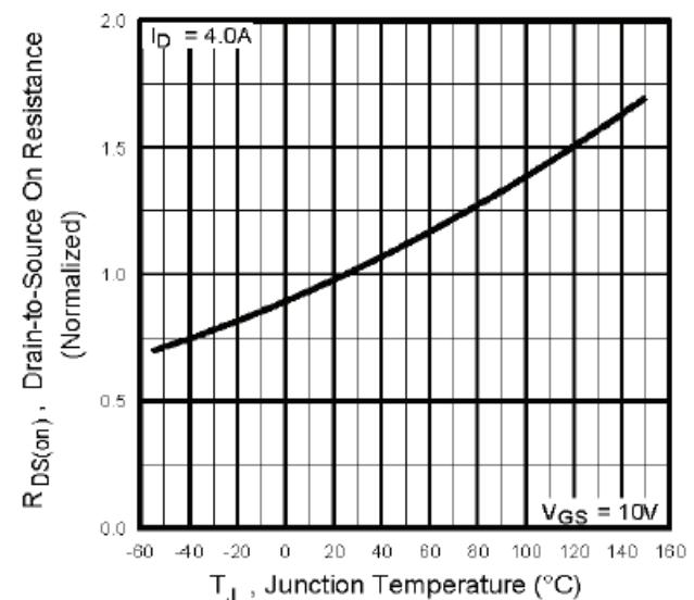
**Fig. 4** Normalized On-Resistance
