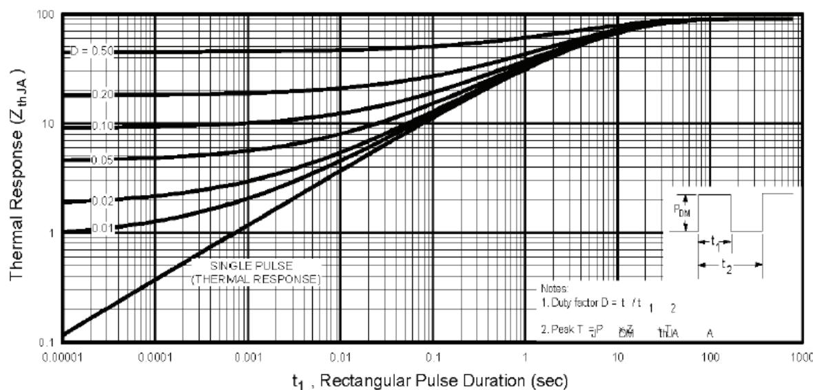
**Fig 23.** Maximum Effective Transient Thermal Impedance, Junction-to-Ambient
