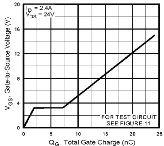
**Fig 6.** Typical Gate Charge vs.
