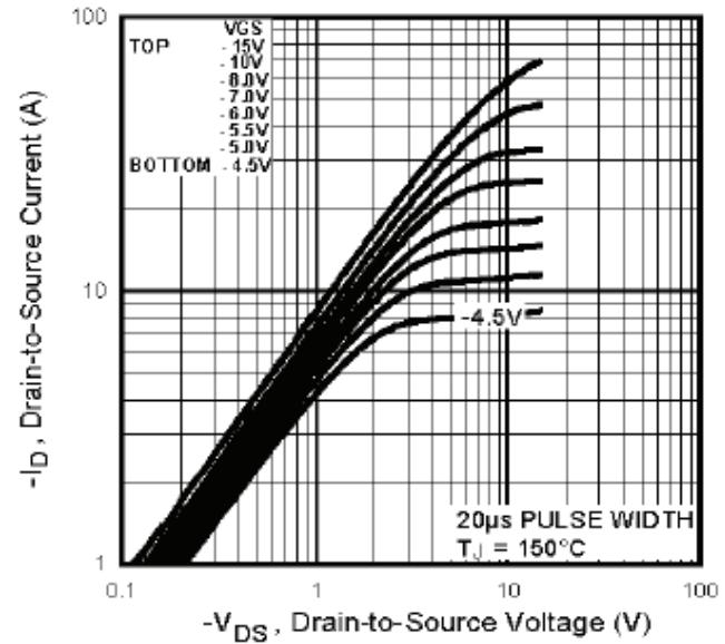
**Fig. 13** Typical Output Characteristics
