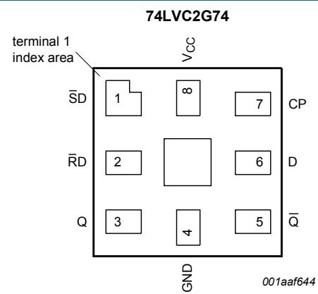
Fig. 6. Pin configuration SOT902-2 (XQFN8)
