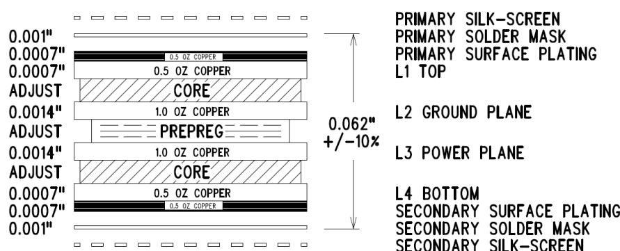
Figure 11. NB3N1200KMNGEVB and NB3W1200LMNGEVB Evaluation Board Layer Stack-Up
