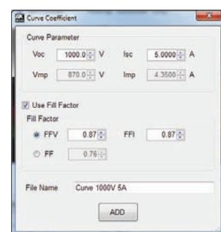
Automatically generate the I-V curve of a solar array in the software by specifying open circuit voltage (Voc), short circuit current (Isc), maximum power voltage (Vmp), and maximum power current (Imp) along with fill factor parameters.
