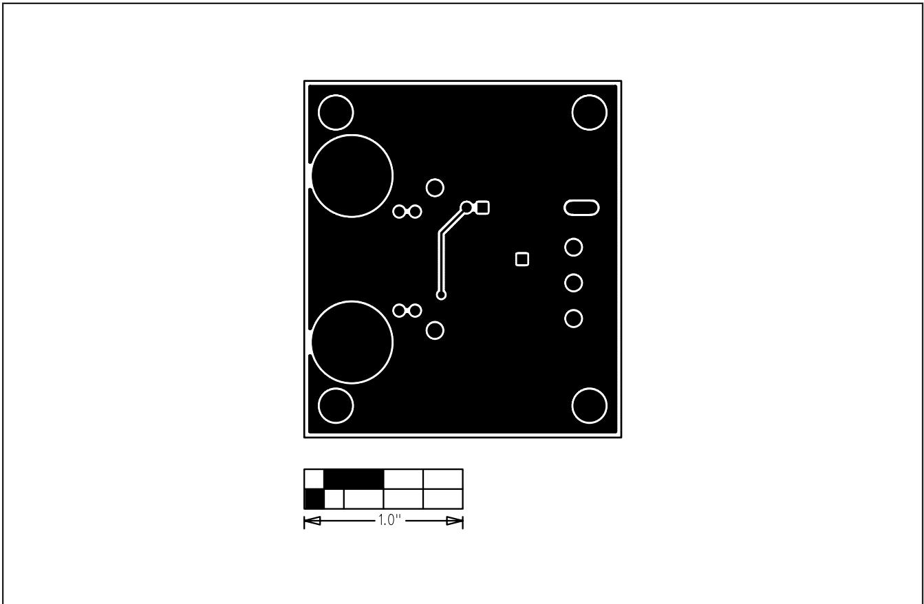
Figure 4. MAX9918 EV Kit PCB Layout—Solder Side
