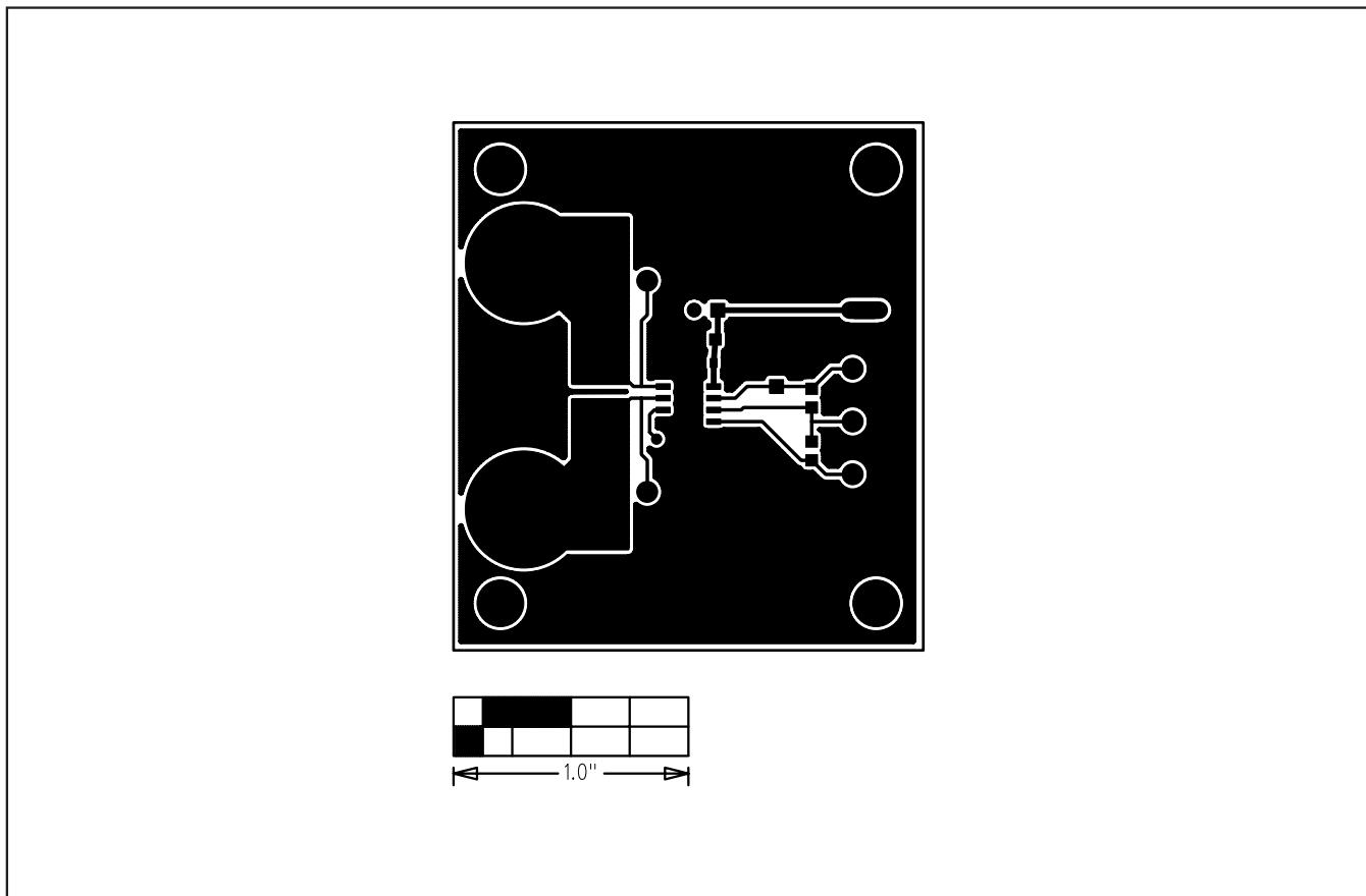
Figure 3. MAX9918 EV Kit PCB Layout—Component Side
