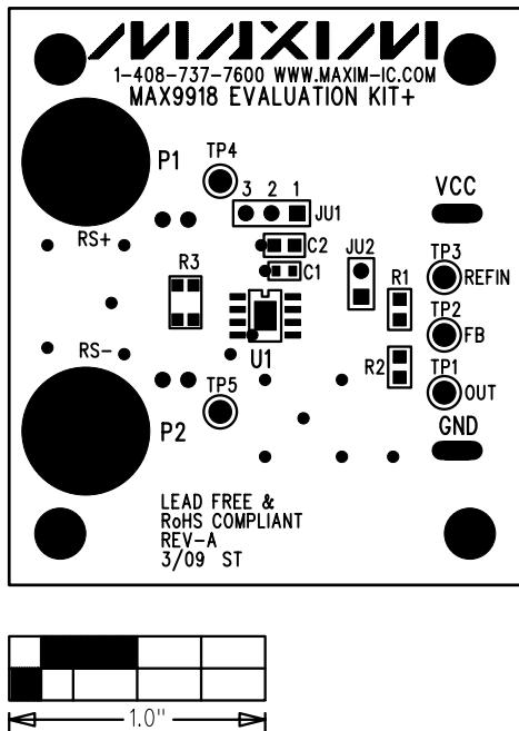
Figure 2. MAX9918 EV Kit Component Placement Guide—Component Side
