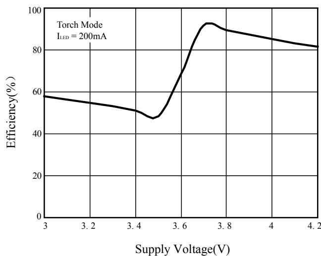
Figure 9 Supply Voltage vs. Efficiency (Torch Mode)
