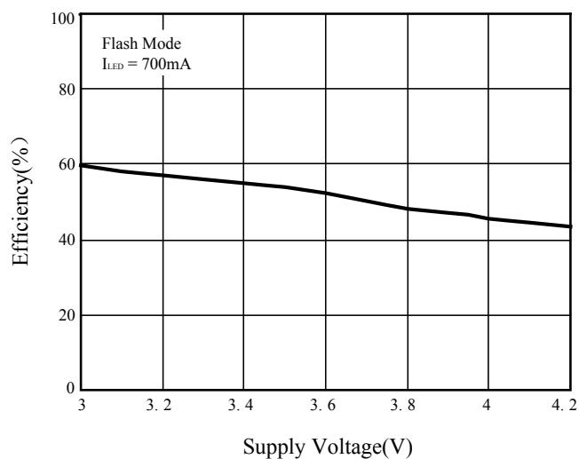
Figure 10 Supply Voltage vs. Efficiency (Flash Mode)
