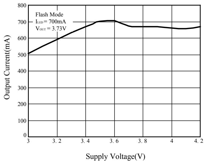
**Figure 4** Supply Voltage vs. Output Current (Flash Mode)
