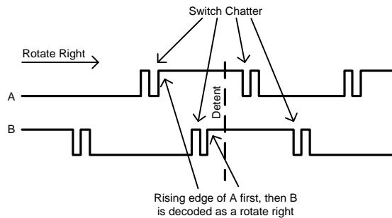
Figure 2. Timing of outputs A and B.
