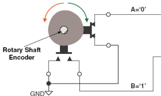
Figure 1. Rotary shaft encoder circuitry.
