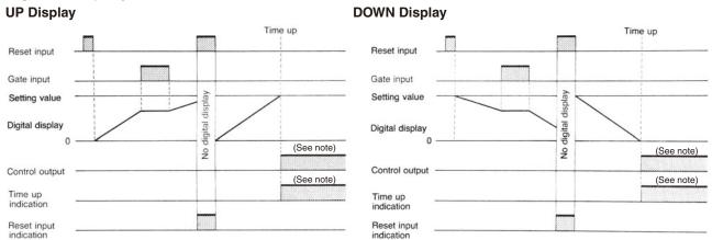
Note: After the set time has elapsed, operation continues according to the mode (N, F, C, R, K, P, or Q).
