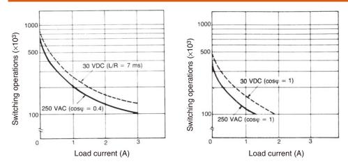
Reference: A maximum current of 0.15 A can be switched at 125 VDC ( $\cos\phi = 1$ ). Maximum current of 0.1 A can be switched if L/R is 7 ms. In both cases, a life of 100,000 operations can be expected. The minimum applicable load is 10 mA at 5 VDC (P reference value).
