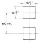
(Horizontally connecting N units)  $\{(n-1) \times 72 + 70 \} \text{ min}$
