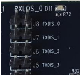
←Headers to manually enable the transmitters
