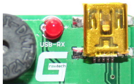
Fig. 10: USB Communication Status LED
