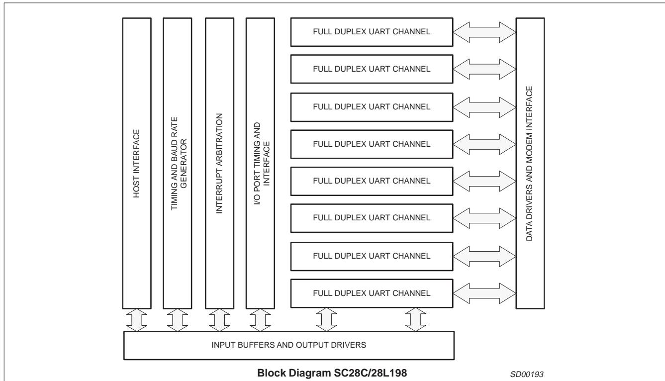
As shown in the block diagram, the Octal UART consists of: an interrupt arbiter, host interface, timing blocks and eight UART channel blocks. The eight channels blocks operate independently, interacting only with the timing, host I/F and interrupt blocks.
