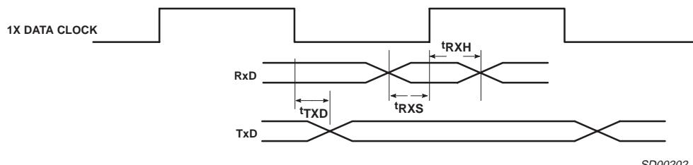
Figure 11. Transmitter and Receiver Timing
