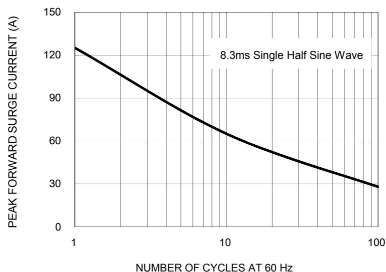
FIG. 3 MAXIMUM NON-REPETITIVE FORWARD SURGE CURRENT
