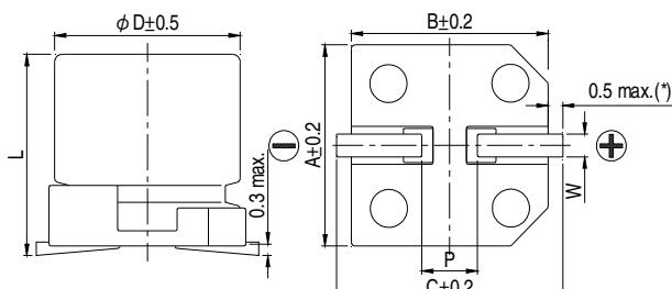
Lead Spacing and Diameter Unit: mm
