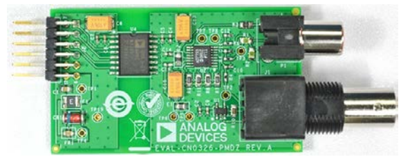
Figure 7. Photo of EVAL-CN0326-PMDZ Board
