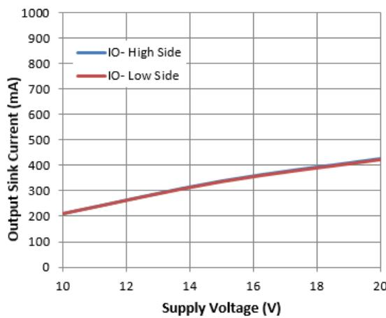
Figure 19. Output Sink Current vs. Supply Voltage
