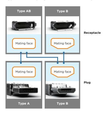
Type A plugs are typically used for connection to "master" devices. Type B plugs are used for connections to "slave" devices. The device itself either features a receptacle that can accept only type B (slave) plugs or both type A and type B plugs (device can function as master or slave). This receptacle is called an "AB" receptacle.
