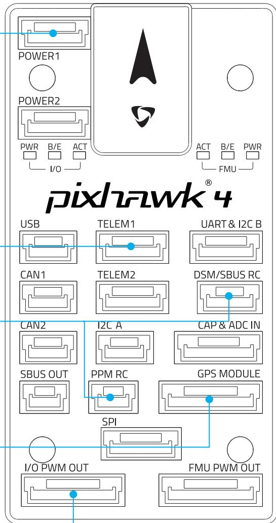
(Optional) Connect a Telemetry Radio to the TELEM port to receive data in Ground Control Station and communicate with the autopilot in flight.
